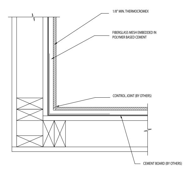
NOTE: All joints of cement board must be treated with 4" fiberglass mesh embedded in polymer based cement.
